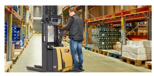
The NSV12P offers a 1.2 tonne capacity, for lighter duties, but is equipped to the same high standard as the other models. The NSV12P(I) is the 1.2 tonne truck fitted with the optional Initial lift feature.
