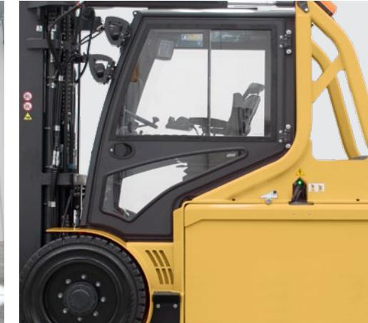
High-capacity batteries and energy-efficient electrical systems give an ideal blend of performance and runtime. Batteries are divided into two parts for easy lateral exchanges using a pallet truck or other forklift. The trucks' low maintenance needs and durability against harsh environments further reduce ongoing costs and downtime.
